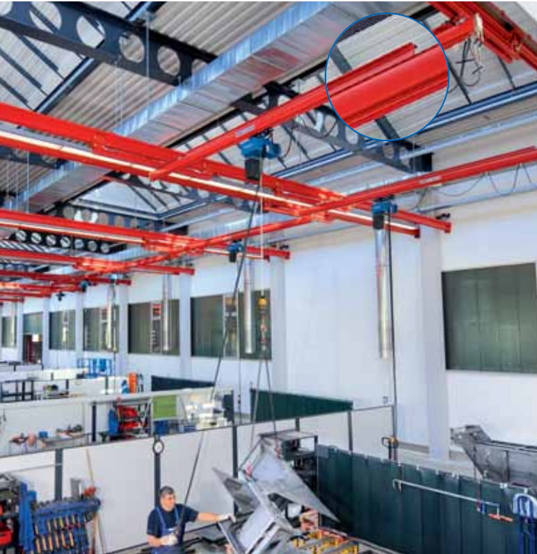
The new KBK II-H profile section replaces the KBK II-T section used until now for Demag suspension cranes (see detail in the circle).
